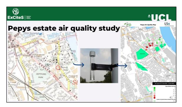
Another example is a study that UCL was involved in 2010, in which after a study of noise at the Pepys Estate in Deptford, south London, we carried out a study of air quality in the area, using a simple device – a diffusion tube, which allows measurement of NO2 level – a pollutant from traffic. IT was possible to show that the area near a local scrapyard is especially polluted.
